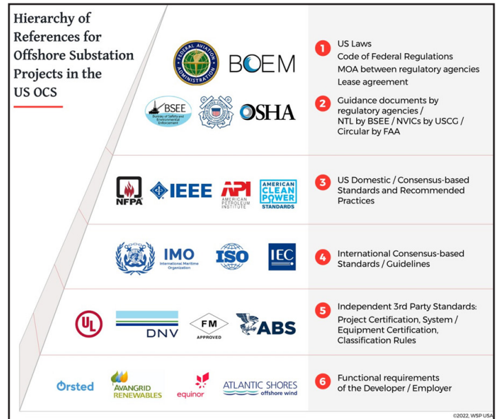
Figure 1. Hierarchy of references for an offshore wind energy substation facility in the US OCS (source: S. Sarada)
